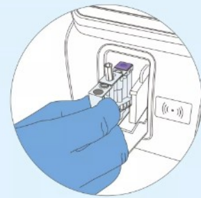
Insert the cartridge into the machine, followed by automatically testing process Result will be displayed in 5 min
